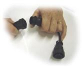
5. Connect the adapter cable to the vehicles diagnostic connector.
