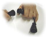
4. Connect the adapter cable to the vehicle diagnostic connector.
